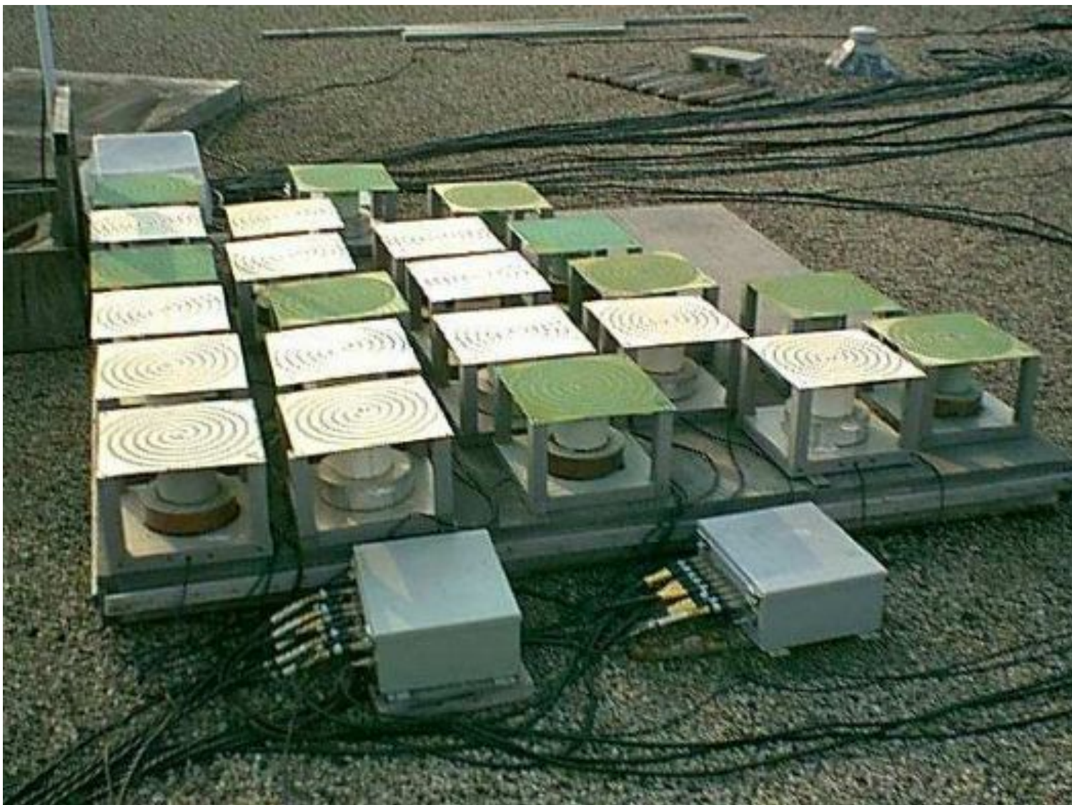
The Ohio Argus Array elements and amplifiers. Note: the calibration source mast is at the upper-left.
